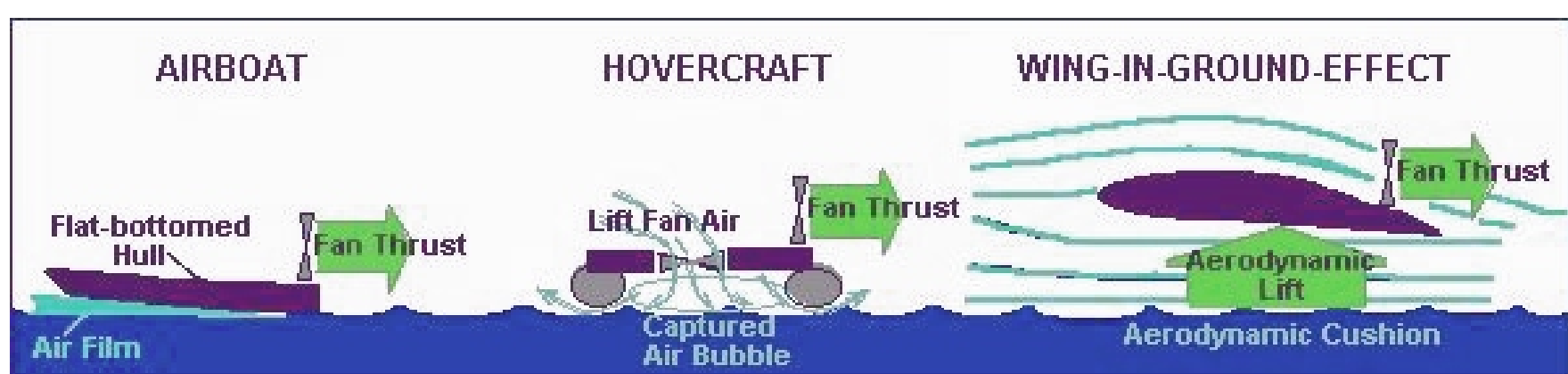
Gambar 7. Perbedaan Airboat , Hovercraft , dan Wing in Ground
